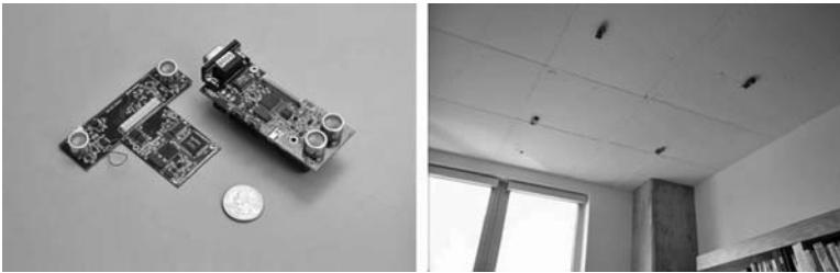
FIGURE 7.8 Cricket tags and example placement of the transmitters ( http://nms.lcs.mit.edu/projects/cricket/ ).
