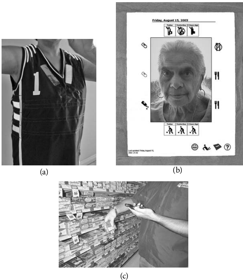
FIGURE 4.1 (a) Augmented jersey from the TeamAwear system. (Courtesy of Mitchell Page.) (b) CareNet display showing information about an elder's activities: (Courtesy of Sunny Consolvo.) (c) Using the AURA system to scan barcodes on items at a grocery store.
