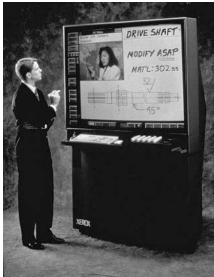
FIGURE 1.5 A commercial version of the Liveboard, sold by Liveworks in the mid-1990s, which evolved out of the original wooden laboratory prototype developed at PARC (see Figure 1.2). (Photo courtesy of PARC, Inc., http://www.parc.com )
