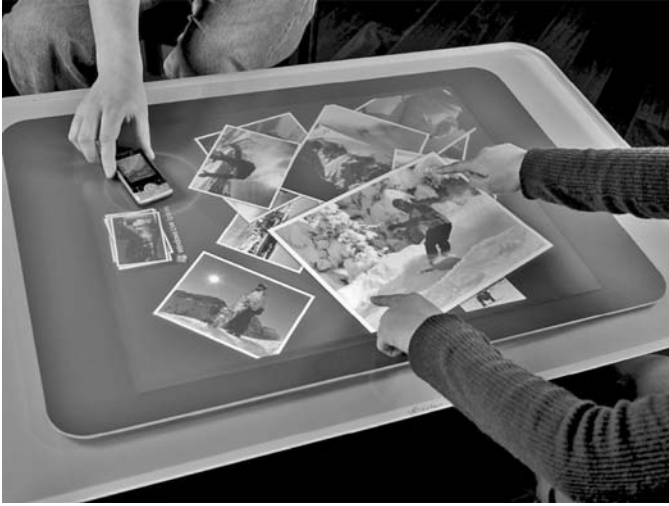
FIGURE 6.7 Microsoft surface detecting device and user touch.
