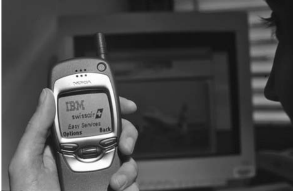
FIGURE 1.6 IBM provided Web-based services for Swissair using WAP on a cell phone to create an electronic boarding pass. (Courtesy of IBM Corp.)
