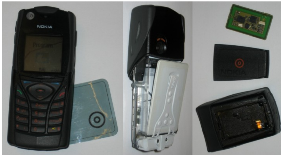
Figure 9.13: Nokia 5140 with RFID transponder sticker, backside showing connector and the Xpress-on RFID Reader Shell back.
