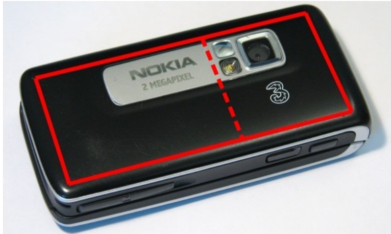
Figure 9.2: Typical back cover antenna coil placements, one with respect to the RF antenna (dashed), displayed on the Nokia 6280.
