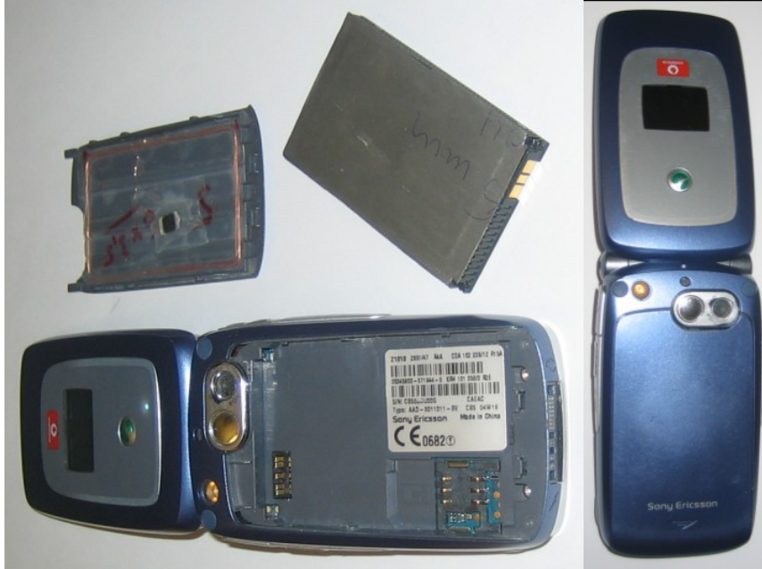
Figure 9.10: Sony Ericsson Z1010 antenna coil implementation, note the \mu -material on the battery.
