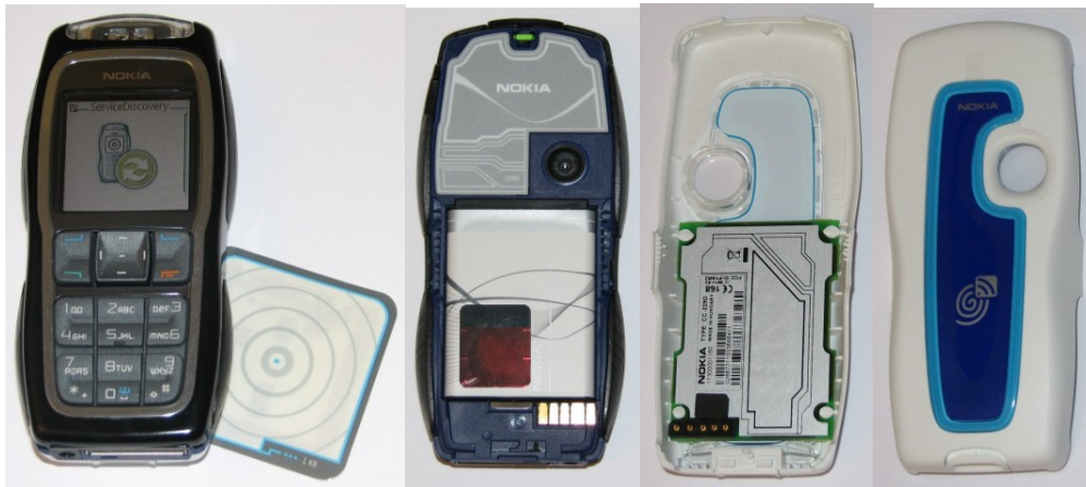
Figure 9.11: Nokia 3220 with NFC transponder sticker, backside showing connector, and the NFC Shell back and front.
