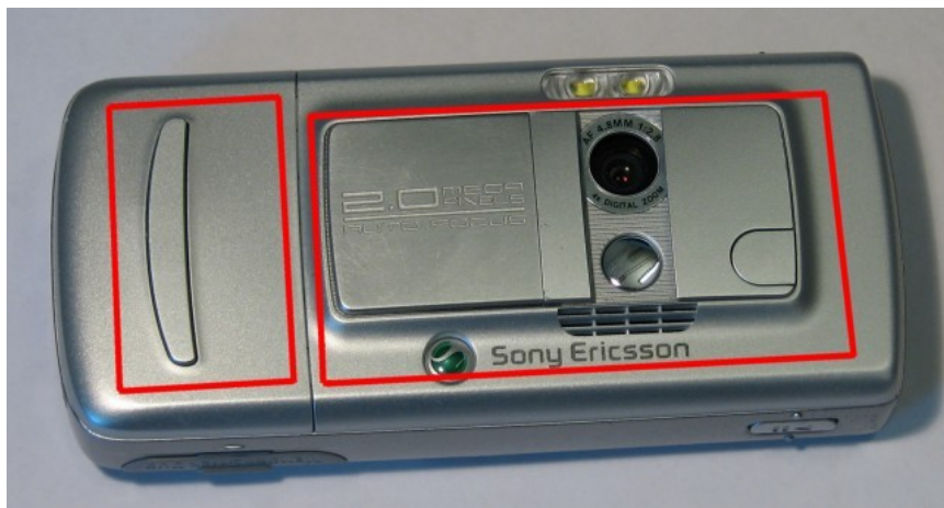
Figure 9.1: The two most common NFC antenna coil placements in commercially available phones, displayed on the Sony Ericsson K750i.
