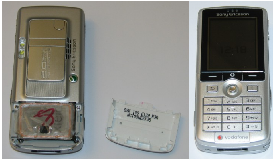
Figure 9.8: Sony Ericsson K750i antenna coil implementation.
