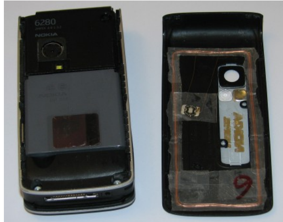
Figure 9.6: Front side view, and NFC implementation on the Nokia 6280.
