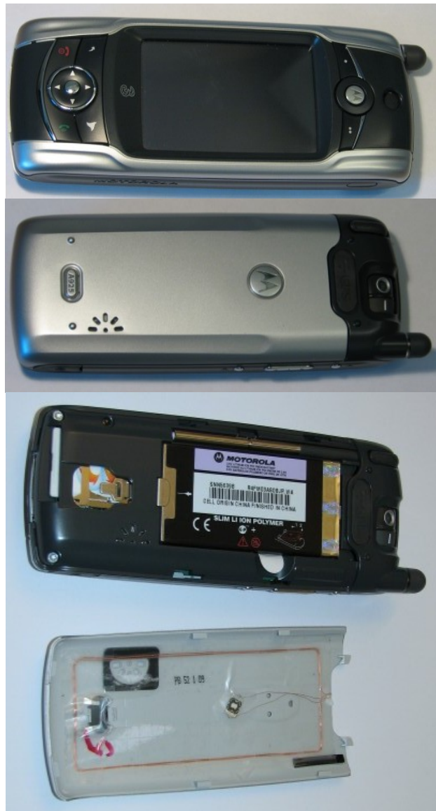
Figure 9.4: The Motorola A925 PDA mobile phone, with optimum antenna coil.
