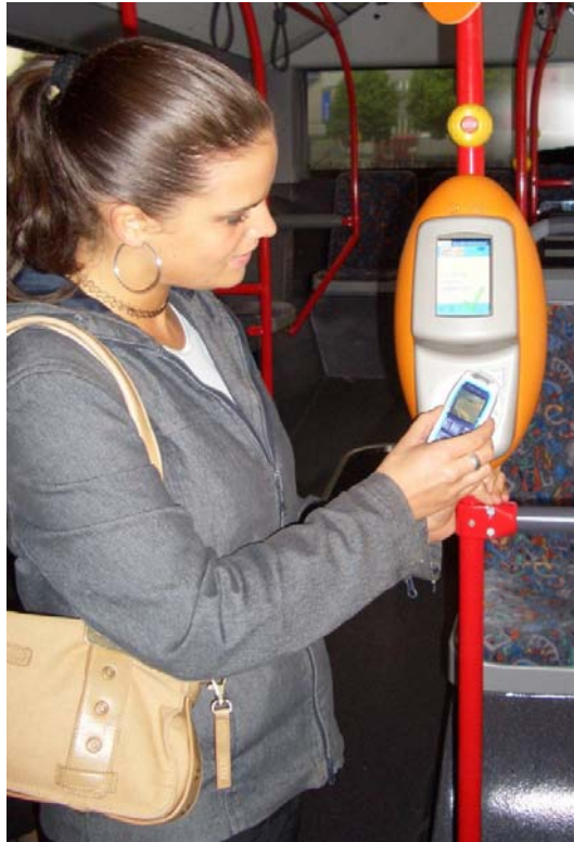
Figure 2.1: Bus ticket electronic payment with the NFC capable Nokia 3220 (reproduced with permission of Rhein-Main-Verkehrsverbund).
