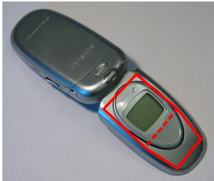
Figure 9.3: Typical antenna coil placement for clamshell models, displayed on the Samsung X460.
