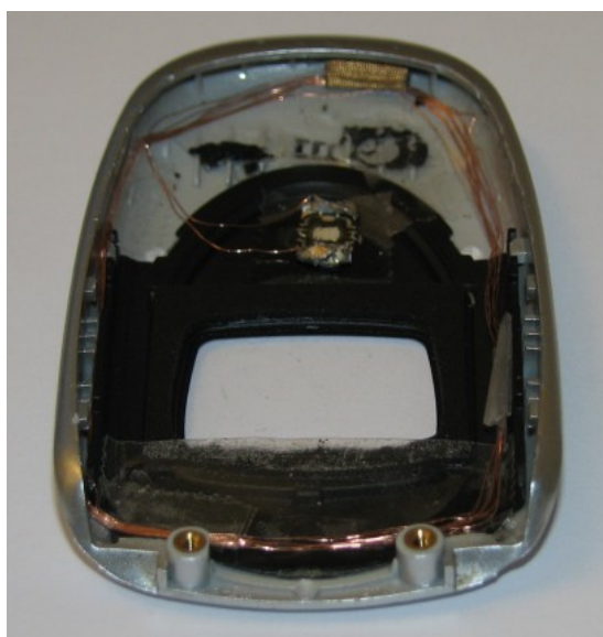
Figure 9.7: Samsung X460 antenna coil implementation.
