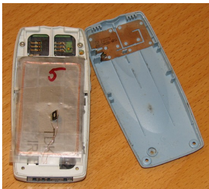
Figure 9.9: Sony Ericsson T65 antenna coil implementation.
