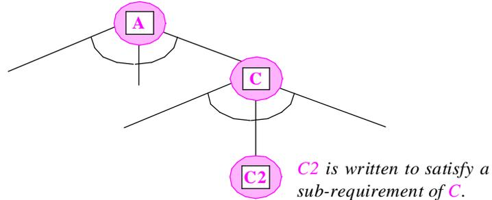
The figure, which shows part of a top-down refinement tree, illustrates this property: *C2* is written to satisfy some sub-requirement of *C*; but the characteristics of *C2* are entirely determined by its immediate context — the needs of *C*. For example, *C* could be a module in charge of analyzing some user input, and *C2* could be the module in charge of analyzing one line (part of a longer input).
