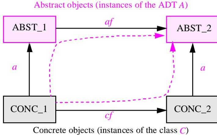
$A$  is an abstract data type, and  $C$  as a class implementing it. For an abstract function  $af$  of the ADT specification — of which we assume for simplicity that it yields a result also of type  $A$  — there will be a concrete feature  $cf$  in the class.
