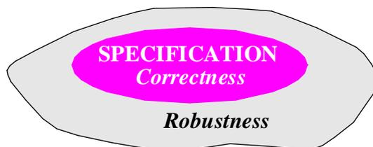
As reflected by the wording of its definition, robustness is by nature a more fuzzy notion than correctness. Since we are concerned here with cases not covered by the specification, it is not possible to say, as with correctness, that the system should “perform its tasks” in such a case; were these tasks known, the abnormal case would become part of the specification and we would be back in the province of correctness.
