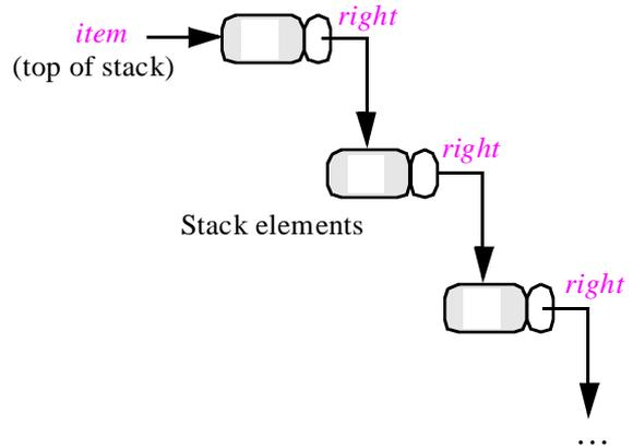
The stack representation, as pictured, takes advantage of the *right* field already present in every *LINKABLE* to link all recycled elements without using any extra space. *LINKABLE* must export *right* and *put\_right* to *STACK\_OF\_LINKABLES* as well as *LINKED\_LIST*.
