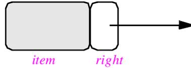
The corresponding class, *LINKABLE*, should be generic, since we want the structure to be applicable to linked lists of any type. The cell value will be given by feature *item*, of type *G*, the generic parameter; this will be an in-place value if the actual generic parameter is expanded, for example for lists of integers or reals, and a reference otherwise. The other attribute, *right*, of type *LINKABLE [G]*, always represents a reference.
