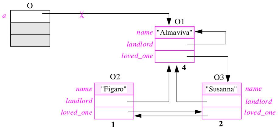
The objects in the right part of the figure, O1, O2 and O3, contain cyclic references to each other; assume that no outside object other than O contains a reference to any of these objects. The corresponding reference counts have been displayed below each object.
