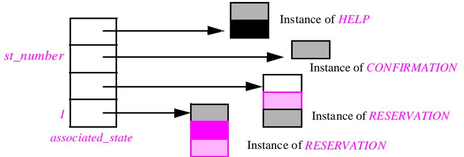
Here is how you build an interactive application. The application will be represented by an entity, say *air\_reservation*, declared of type *APPLICATION*. You must create the corresponding object:
