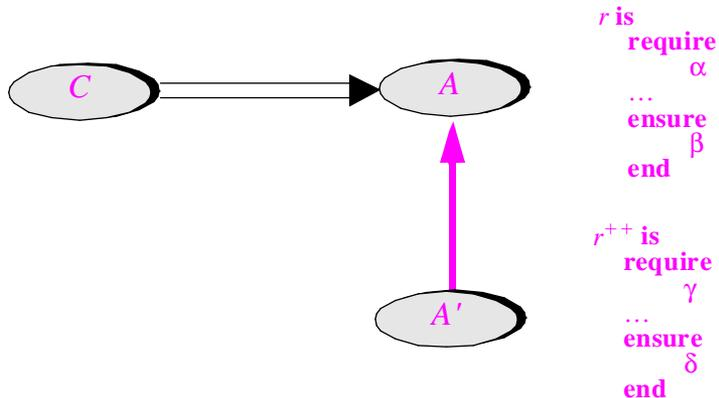
Assume that a new class  $A'$  inherits from  $A$  and redeclares  $r$ . How, if at all, can it change the precondition  $\alpha$  into a new one  $\gamma$  and the postcondition  $\beta$  into a new one  $\delta$ ?
