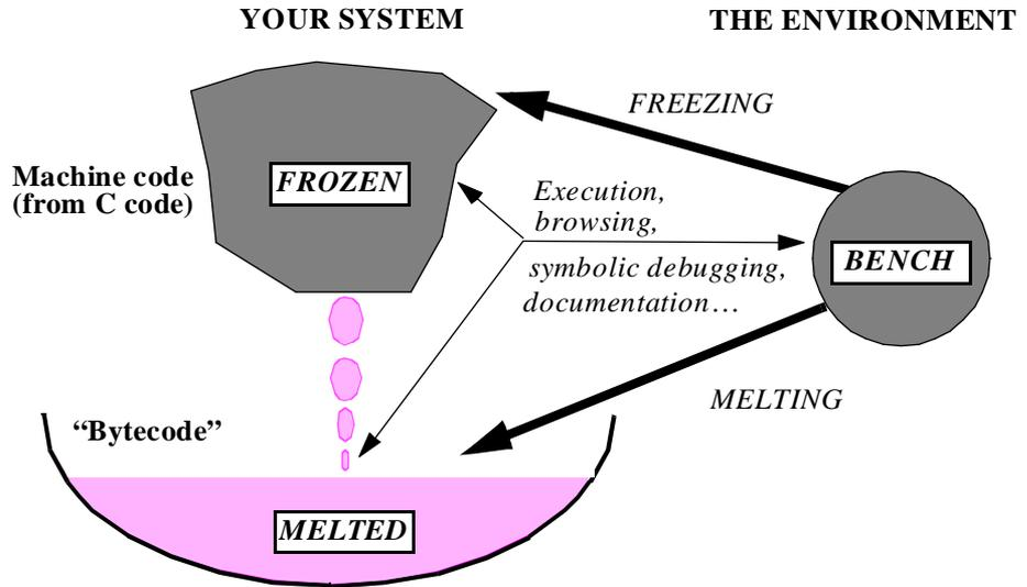
The tricky part (for the compiler implementers) is of course to make sure that the various components can work together, in particular that frozen code can call melted elements — even though it was not known, at freezing time, that they would later be melted! But the result is definitely worthwhile:
