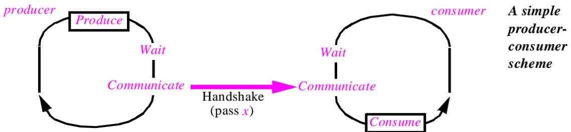
Communication occurs when both processes are ready for each other; this is sometimes called a *handshake* or *rendez-vous*. The design of synchronization mechanisms — enabling us in particular to express precisely the instructions to “*Make it known that process is ready*” and “*Wait for process to be ready*” — has been a fertile area of research and development for several decades.
