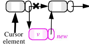
To insert a new item of value *v*, we must create a cell of type *LINKABLE* [*G*]; the actual insertion is carried out by the secret procedure *put\_linkable\_right*, which takes a *LINKABLE* as argument (and chains it to the cursor item using the *put\_right* procedure of class *LINKABLE*.) This procedure performs the appropriate reference manipulations.
