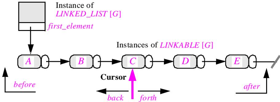
We permit the cursor to be on a list element (if any), or one position to the left of the first, in which case the boolean query *before* will return true, or one position to the right of the last, making *after* true.
