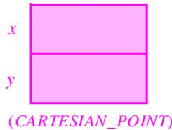
If  $p1$  is the point shown, getting its  $x$  or its  $y$  simply requires looking up the corresponding field in this structure. Getting  $\rho$  or  $\theta$ , however, requires a computation: for  $\rho$  we must compute  $\sqrt{x^2 + y^2}$ , and for  $\theta$  we must compute  $\arctg(y/x)$  with non-zero  $x$ .
