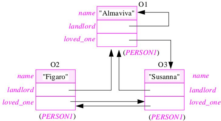
The Persistence Closure principle stated that any mechanism that stores O1 must also store all the objects to which it refers, directly or indirectly; otherwise when you retrieve the structure you would get a meaningless value (“*dangling reference*”) in the *loved\_one* field for O1.
