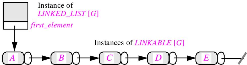
This representation makes insertion or deletion fast if you have a reference to the linkable immediately to the left of the operation's target: a few reference manipulations will do, as shown here for the deletion of the third element.
