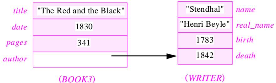
the object-oriented model made it easy to access indirect properties of an object, such as *redblack.author.birth\_year* (yielding *1783* if *redblack* is attached to the object on the left of the figure). A relational description will not be able to represent the reference field *author*, whose value is the denotation of another object.
