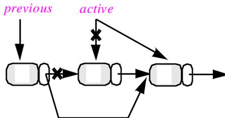
The routine looks trivial; but this is only thanks to the technique of keeping the left sentinel around as a physical object, avoiding constant tests of the form *previous /= Void* and *first\_element /= Void*. It is worth considering the more complicated and less efficient routine body that we would have obtained without this simplification:
