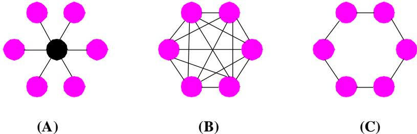
More precisely, if a system is composed of  $n$  modules, then the number of intermodule connections should remain much closer to the minimum,  $n-1$ , shown as (A) in the figure, than to the maximum,  $n(n-1)/2$ , shown as (B).
