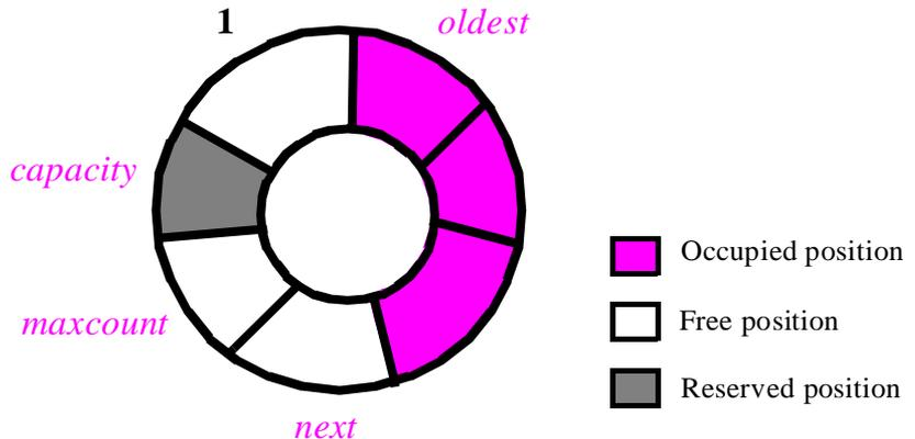
The procedure *put* used by a producer to add an item  $x$  will be implemented as  $\text{representation.put}(x, \text{next}); \text{next} := (\text{next} \parallel \text{maxcount}) + 1$
