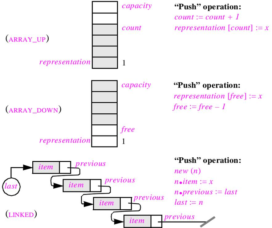
The figure illustrates three of the most common representations. Each has been given a name for ease of reference:
