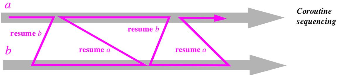
This is all strictly sequential and meant to be executed on a single process (task) of a single computer. But the ideas are clearly drawn from concurrent computation; in fact an operating system running on a single CPU will internally use a coroutine-like mechanism to implement such schemes as time-sharing, multitasking and multithreading.
