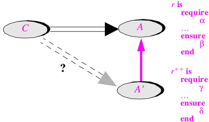
the assertions of the redeclared version,  $\gamma$  and  $\delta$ , if different from  $\alpha$  and  $\beta$ , are more favorable to the clients, in the sense explained earlier (weaker precondition, stronger postcondition). But a client of *A* which uses *A'* through polymorphism and dynamic binding cannot make good use of this improved contract, since its only contract is with *A*.
