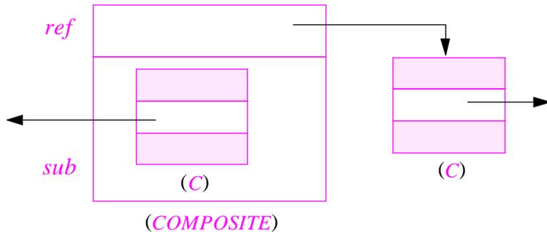
The *ref* field is a reference attached to an instance of *C* (or void). The *sub* field (which cannot be void) contains an instance of *C*.
