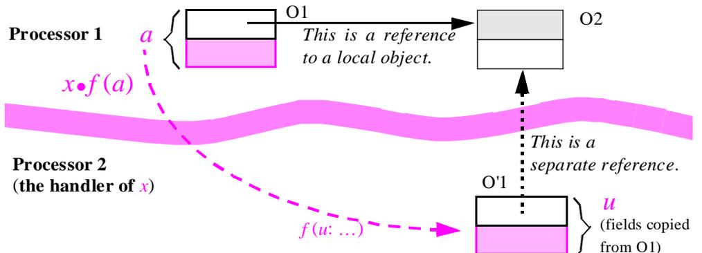
The figure illustrates the case in which the formal argument  $u$  is itself expanded. Then the attachment is simply a copy of the fields of the object O1 onto those of the object O'1 attached to  $u$ . Permitting O1 to contain a reference would produce a traitor field in O'1. The problem would also arise if O1 had a subobject with a reference; hence the mention “directly or indirectly” in the rule.
