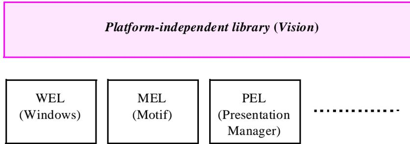
To make things more concrete the figure shows the names of the corresponding components in ISE's environment, but the idea is applicable to any graphical library. At the top level (*Vision*) there is a portable graphical library; at the bottom level you find specialized libraries, such as *WEL* for Windows, adapted to one platform only.
