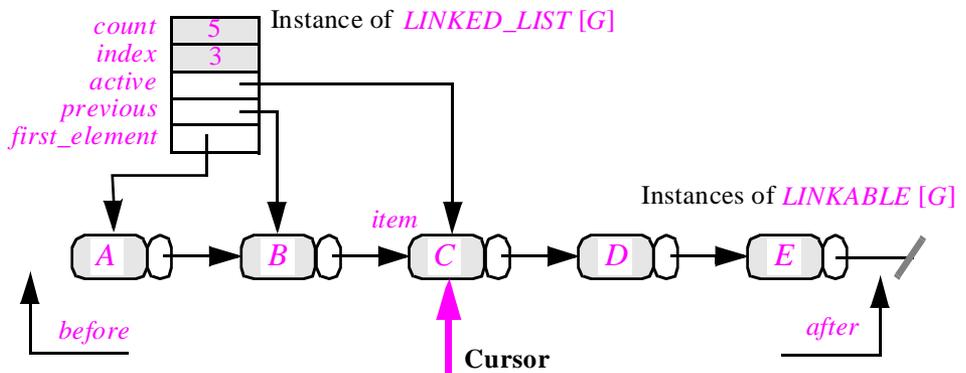
Along with *first\_element* it will be useful to keep two references in the list header, enabling us to perform insertions and deletions efficiently: *active*, attached to the cursor item at cursor position, and *previous* attached to the previous one.
