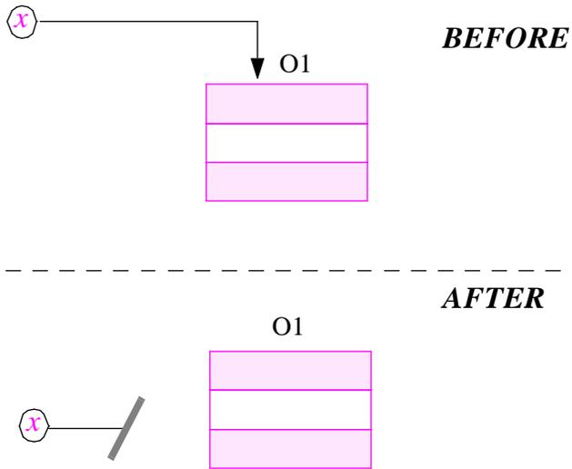
The comment made in the general discussion of reference assignment is worth repeating here: the assignment of *Void* to *x* has no immediate effect on the attached object (O1 in the figure); it simply cuts the link between the reference and the object. It would be incorrect to understand it as freeing the memory associated with O1, since some other reference may still be attached to O1 even after *x* has been de-attached from it. See the discussion of memory management in the next chapter.
