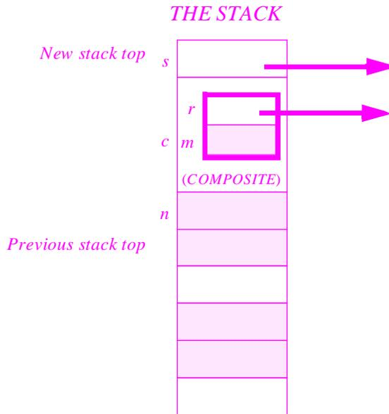
The three new values are an integer  $n$ , which does not affect the problem of object management (since it will disappear when the procedure terminates, and does not refer to any other object); a reference  $s$ , which is an example of category **O1**; and an object  $c$  of type *COMPOSITE*. This object is itself stack-based and its allocated memory may be reclaimed on procedure termination; but it contains a reference field for  $r$ , which is an example of category **O2**.
