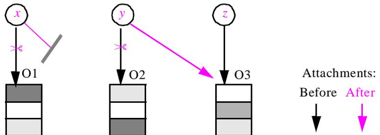
The principal causes of detachment are the following, assuming  $x$  and  $y$ , entities of reference type, were initially attached to objects  $O1$  and  $O2$ . The figure illustrates cases **D1** and **D2**.
