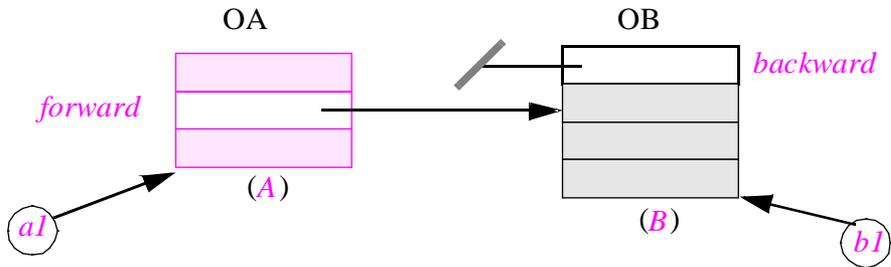
The invariant is violated on OA! This object is now linked to OB, but OB is not linked to OA since its *backward* field is void. (A call to *b1.attach (...)* could also have linked OB to an instance of *A* other than OA, which would be equally incorrect.)
