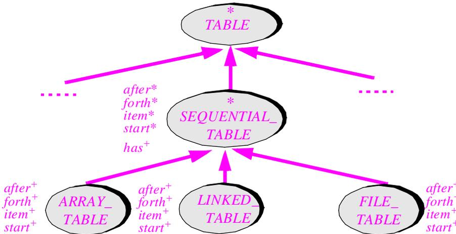
The most general class, *TABLE*, is fully or almost fully deferred, since at that level we may specify a few features but not provide any substantial implementation. Among the variants is *SEQUENTIAL\_TABLE*, representing tables in which elements are inserted sequentially. Examples of sequential tables include array, linked list and sequential file implementations. The corresponding classes, in the lowest part of the figure, are effective.
