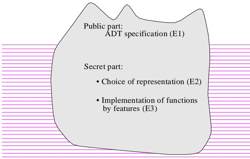
If the module is a class coming from an ADT as outlined above, the answer is clear: of the three parts involved in the transition, *E1*, the ADT specification, is public; *E2* and *E3*, the choice of representation and the implementation of the ADT functions in terms of this representation, should be secret. (As we start building classes we will encounter a fourth part, also secret: auxiliary features needed only for the internal purposes of these routines.)
