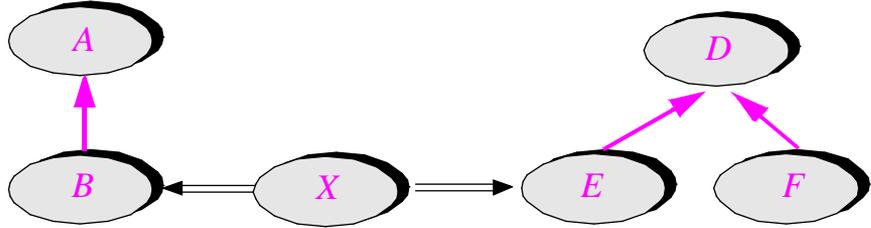
When *B* gets abstracted into *A*, or the features of *E* get factored with those of *F* into *D*, a class *X* that is a client of *B* or *E* (in the figure it is a client of both) will in many cases not feel any effect from the change. The ancestry of a class does not affect its clients if they are simply applying the features of the class on entities of the corresponding type. In other words, if *X* uses *B* and *E* as suppliers under the scheme
