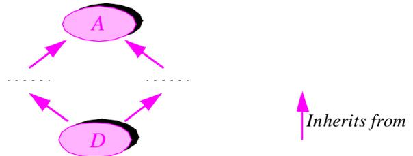
In such a case the language must provide precise rules defining what happens to features inherited repeatedly from the common ancestor, *A* in the figure. As the discussion of repeated inheritance will show, it may be desirable for a feature of *A* to yield just one feature of *D* in some cases (*sharing*), but in others it should yield two (*replication*). Developers must have the flexibility to prescribe either policy separately for each feature.
