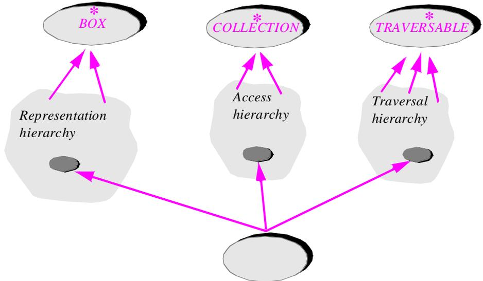
But then we realized that it was inappropriate to keep *BOX*, *COLLECTION* and *TRAVERSABLE* separate: they all needed a few common features, in particular *has* (membership test) and *empty* (test for no elements). This clearly indicated the need for a common ancestor — *CONTAINER*, where these common features now appear. Hence a structure that was initially designed as pure multiple inheritance, with three disjoint
