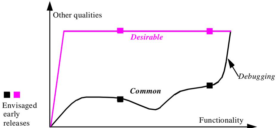
The bottom curve (black) is all too common: in the hectic race to add more features, the development loses track of the overall quality. The final phase, intended to get things right at last, can be long and stressful. If, under users' or competitors' pressure, you are forced to release the product early — at stages marked by black squares in the figure — the outcome may be damaging to your reputation.
