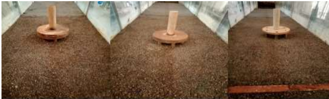
Figure 12: Pile cap above bed level submerged in water having different thicknesses.
