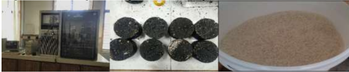
Figure 1: Indirect test apparatus, Marshall Specimen, Sasobit
