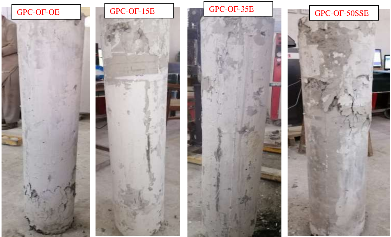
Figure 5 Failure modes of GPC specimens
