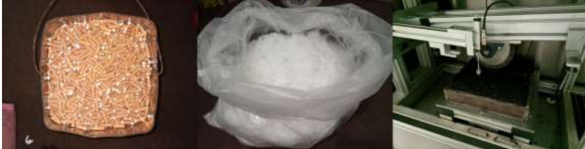
Figure 1: Cigarette Butts, Cigarette Butt fibers, Wheel Tracker sample
