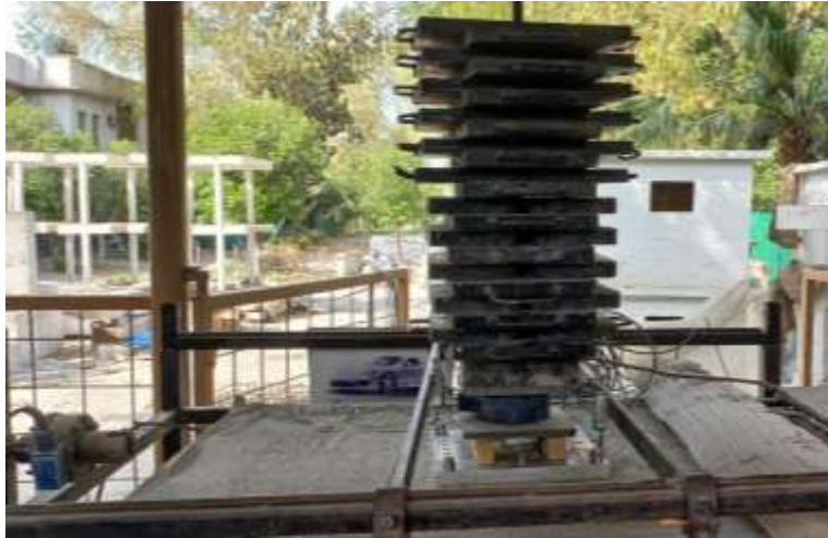
Figure 3: Overall arrangements for vertical load application
