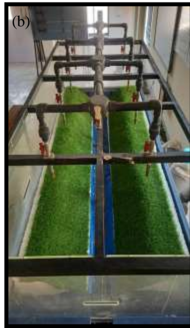
Fig. 2: (a) No vegetation model, (b) flexible vegetation model, (c) mixed vegetation model
