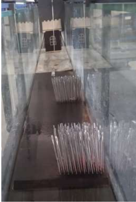
Fig: 2.1: Experimental models; (a,c) vegetation place in the channel, (b) USB Accelerometer and (d) House model
