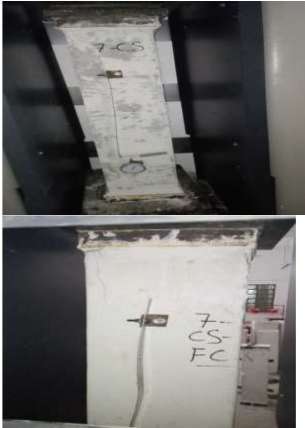
Figure 3: Specimens in compression testing machine
