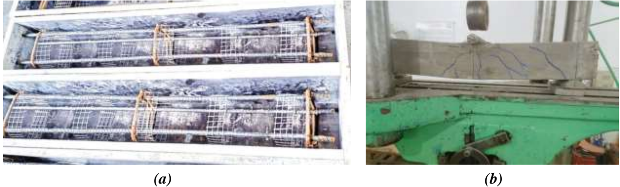
Figure 5: (a) 1.5" Wide Mesh Strip (b) Actual Laboratory Test Setup
