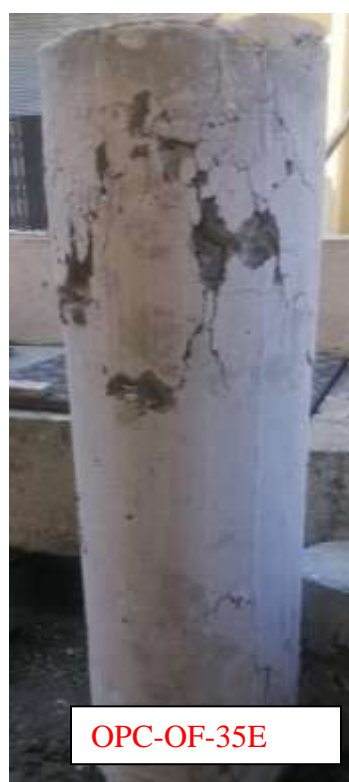
Figure 4 Failure mode of OPC specimens
