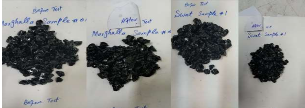
Figure 6: Stripping and Coating Samples before and after test
