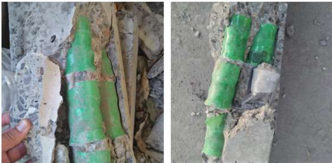
Figure 8: Pictures Showing the weak bond of Plastic Bottles with concrete
