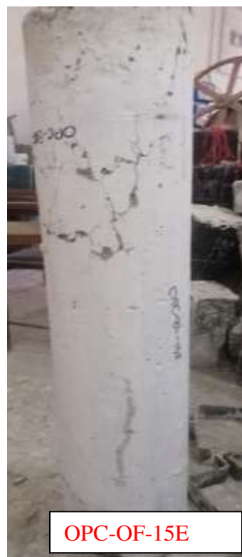
Figure 4 Failure mode of OPC specimens
