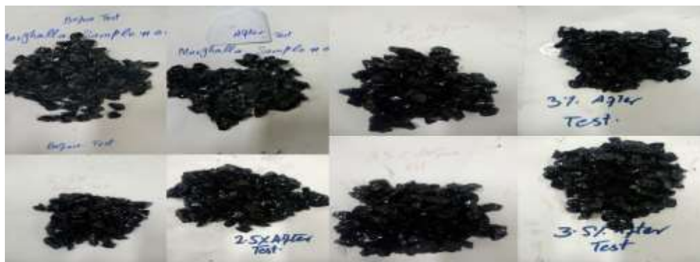
Figure 6: Stripping and coating Test sample before and after test
