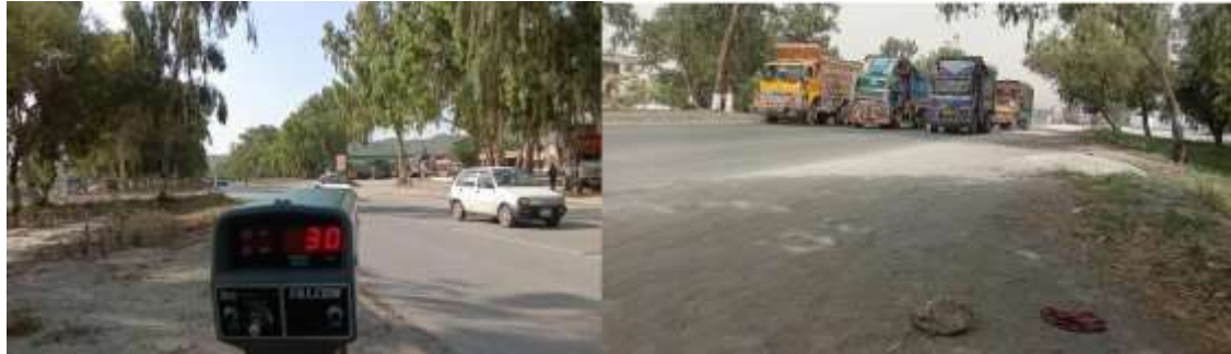
Figure II: Measurement of spot speed and traffic composition
