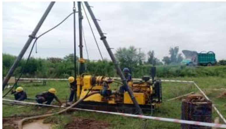
Figure 1: Straight rotary rig during the drilling process
