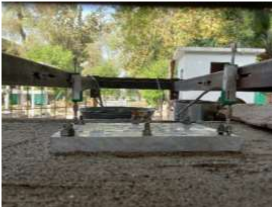
Figure 1: Installation of Raft and LVDTs after Pluviation
