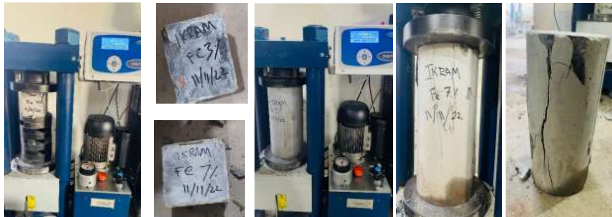
Figure 2: Compression Testing of Specimens
