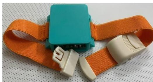
Figure 1: Complete Module having 3D printed body, PCB, ESP controller, MPU 6050 and BMS.
