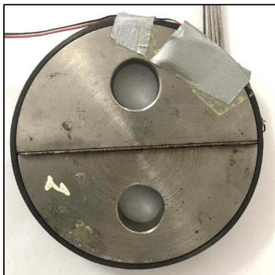
*Figure 3b. Sample wrapped around split disk*
