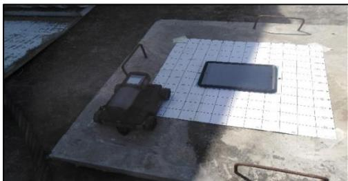
*Figure 2: Calibration of GPR*
