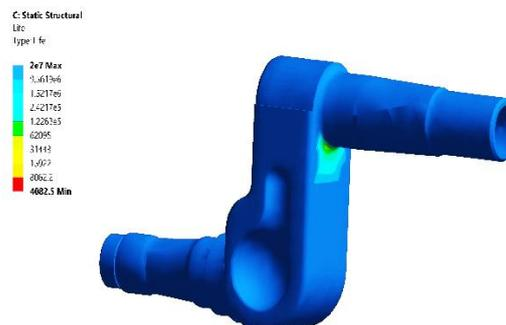
Figure 4: Fatigue Life of Balance arm for smooth terrain
