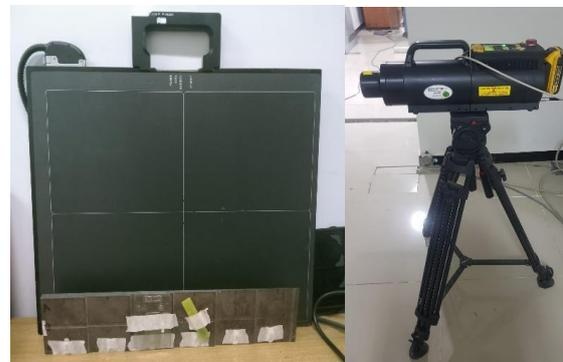
*Figure 2: Leonardo DR system with wireless flat panel detector and the generator*
