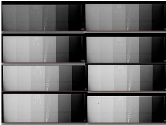
**Figure 7:** Digital radiography images of a step wedge, taken with pulse settings ranging from 1 to 8, demonstrating varying exposure levels
