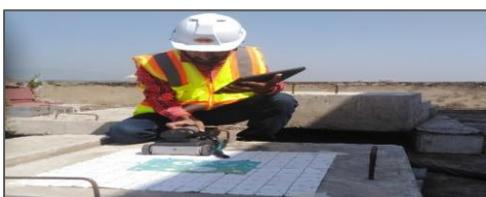
*Figure 3: Scanning of Concrete block using GPR*
