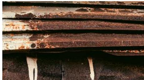
*Figure 1: Pitting corrosion [1]*
