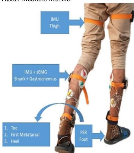
Figure 4: Completer hardware DAQ system based on Conceptual Sketch
