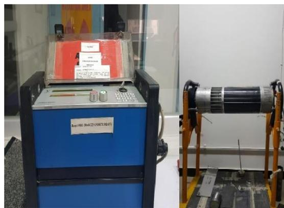
*Figure 6: Model 225 ANDREX SMART (machine used for conventional radiography)*
