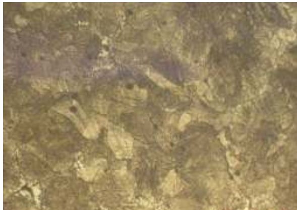
Figure 4.11: Microstructure: tempered martensite X350
