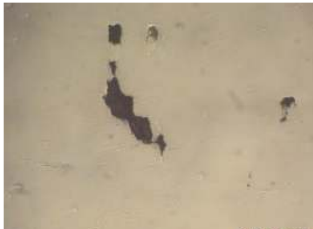
Figure 4.10: Oxide type Inclusions: as-polished specimen X100
