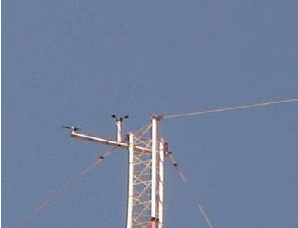
Figure 3.1: Top Mounted Boom Anemometer with Vane
