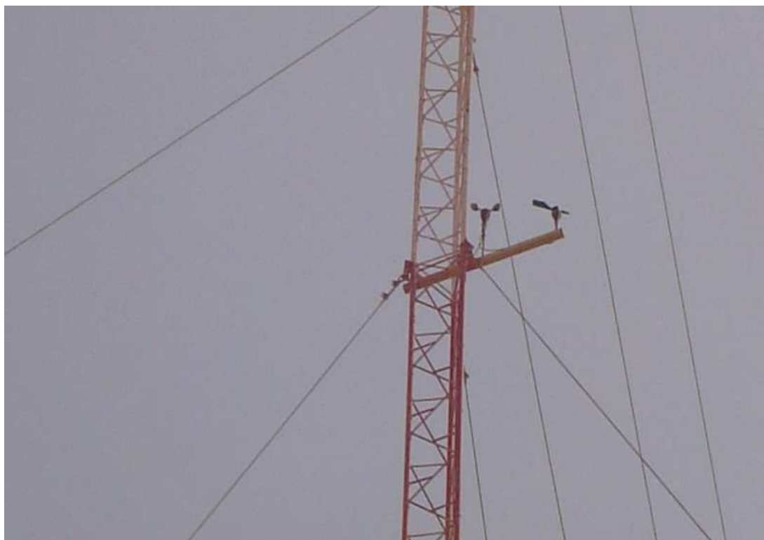
Figure 3.4: Anemometer mounted with Wind Vane on 30 m high boom
